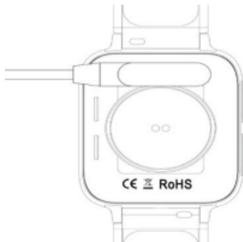
\*Please note that the two contacts of the charger cannot contact the conductor at the same time, which will cause the circuit to burn.
